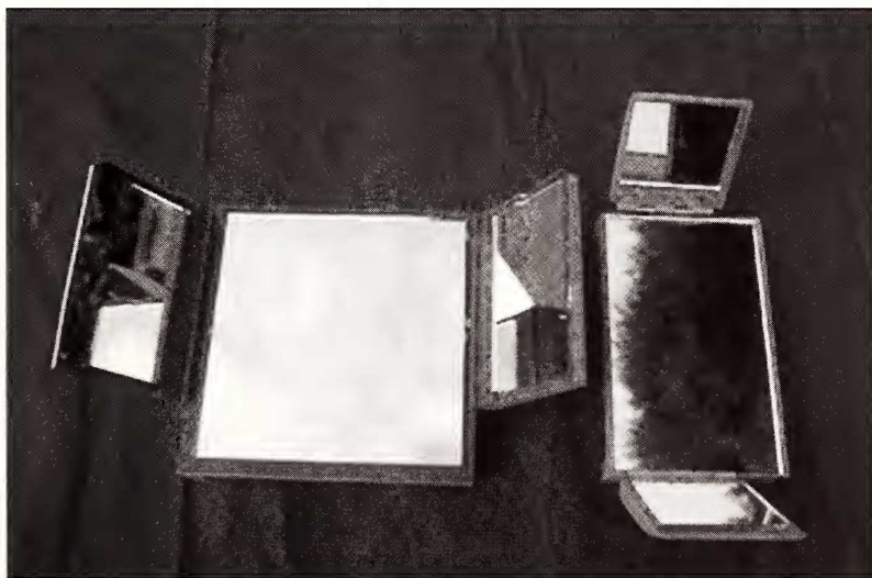
Figure 4. Articulated Mirror Assemblies.
